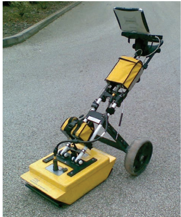
Fig. 62 Example of GPR scanner equipment.
